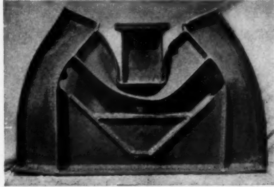
FIG. 12. SHOCK TEST PIECE AFTER TESTING
